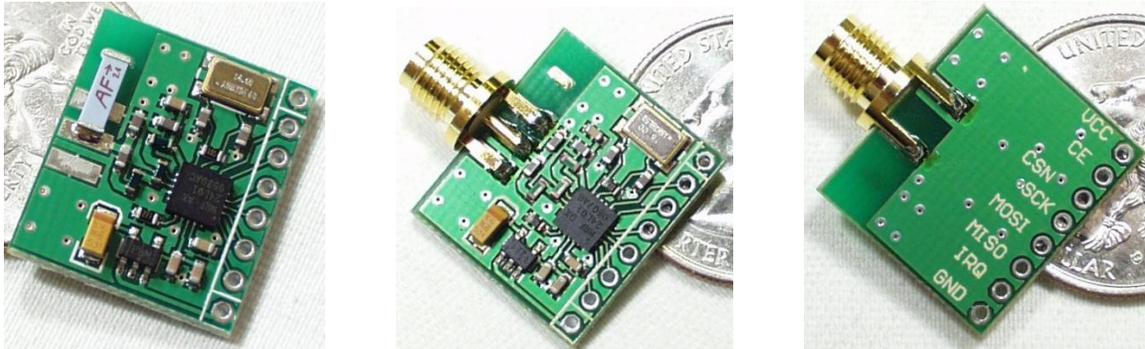
**Figure 1.** Left to right: MiRF-v2 top, MiRF-v2 RP-SMA top and bottom (pics from [www.sparkfun.com](http://www.sparkfun.com))
