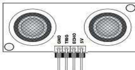
Fig.5 Ultrasonic Sensor [10]
