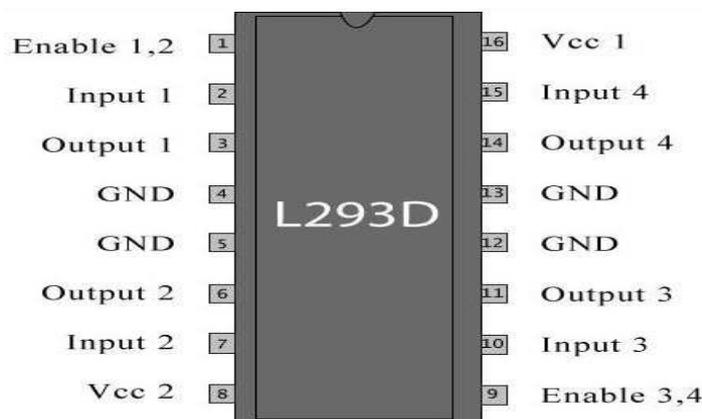
**Fig.8 Pin configuration of L293D [13]**
