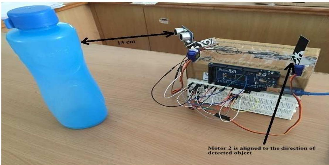
Fig.11 Hardware Realization of the proposed system
