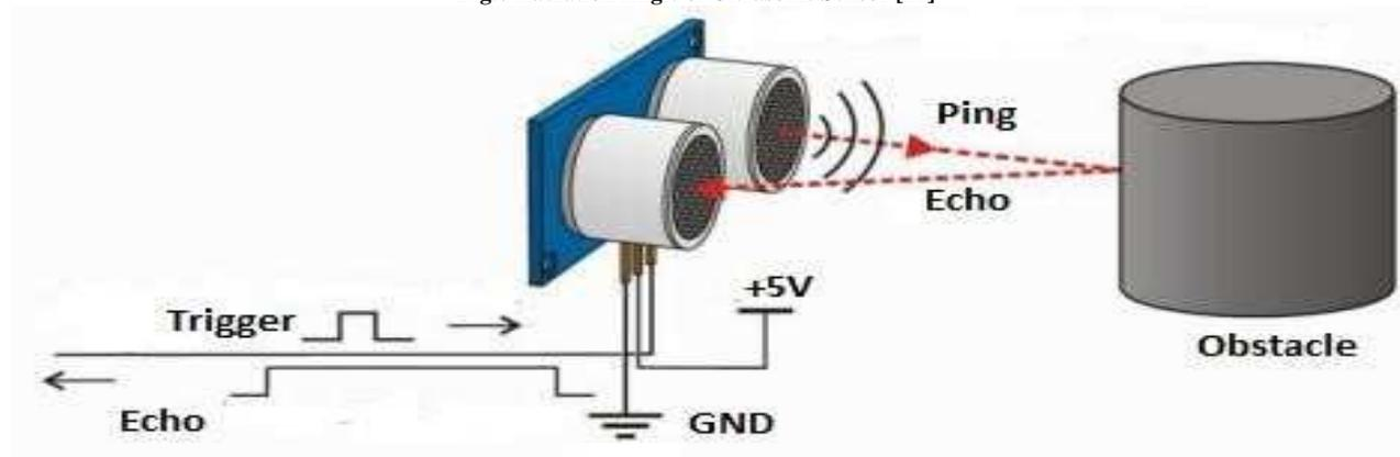
**Fig.7 Working of Ultrasonic Sensor [12]**
