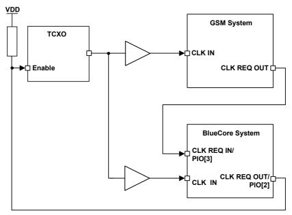
Figure 11.32: Example TXCO Enable OR Function
