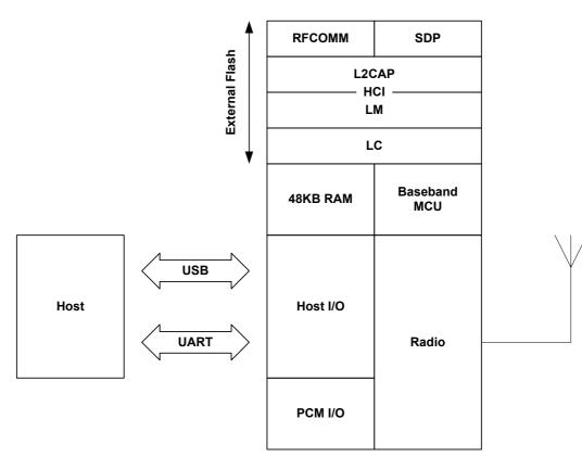
Figure 9.2: BlueCore RFCOMM Stack
