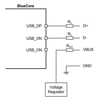
Figure 11.16: USB Connections for Bus-Powered Mode
