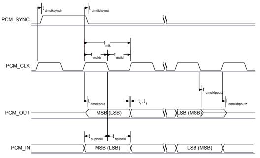
Figure 11.28: PCM Master Timing Short Frame Sync
