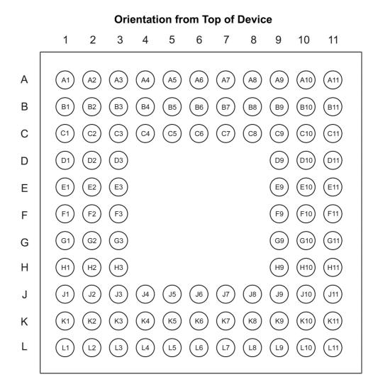
Figure 3.2: BlueCore4-External 6 x 6mm Device Pinout (BC417143B-IRN-E4)
