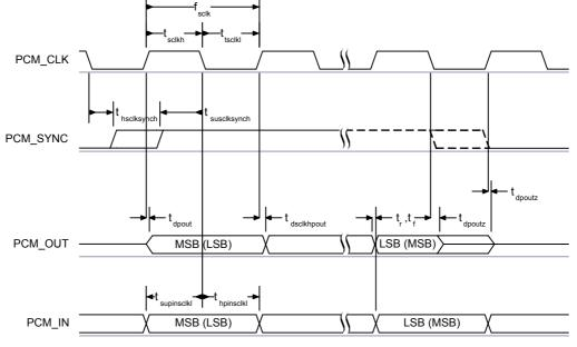
Figure 11.29: PCM Slave Timing Long Frame Sync
