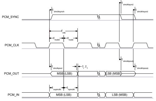
Figure 11.27: PCM Master Timing Long Frame Sync
