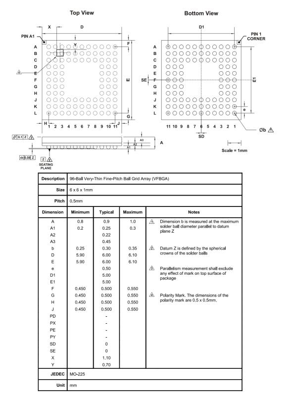
Figure 13.2: BlueCore4-External 96-Ball VFBGA Package Dimensions
