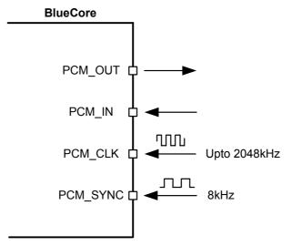
Figure 11.21: BlueCore4-External as PCM Interface Slave
