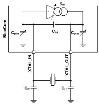
Figure 11.5: Crystal Driver Circuit
