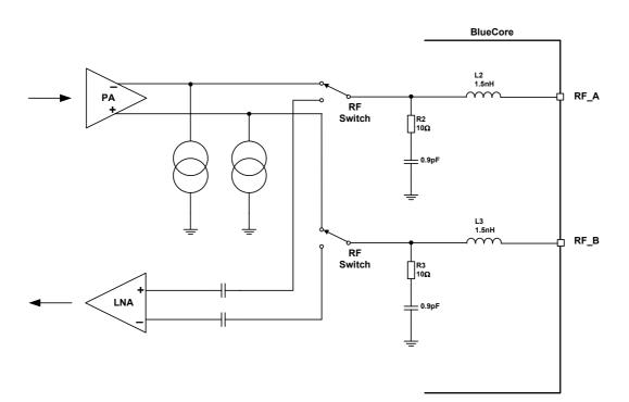
Figure 11.1: Circuit TX/RF\_A and TX/RF\_B
