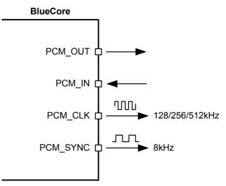
Figure 11.20: BlueCore4-External as PCM Interface Master
