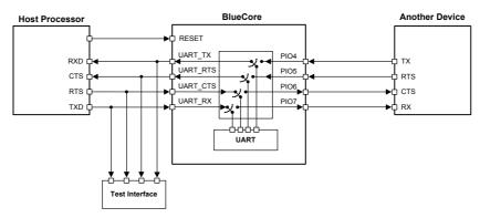
Figure 11.14: UART Bypass Architecture
