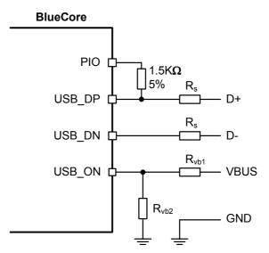
Figure 11.15: USB Connections for Self-Powered Mode
