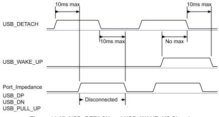
Figure 11.17: USB\_DETACH and USB\_WAKE\_UP Signal
