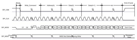
Figure 11.18: Write Operation
