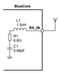
Figure 11.2: Circuit RX\_IN
